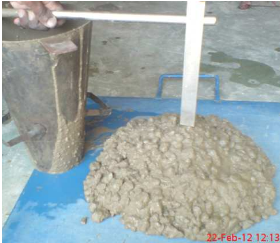
Concrete Slump @ 12:13 = 185mm
