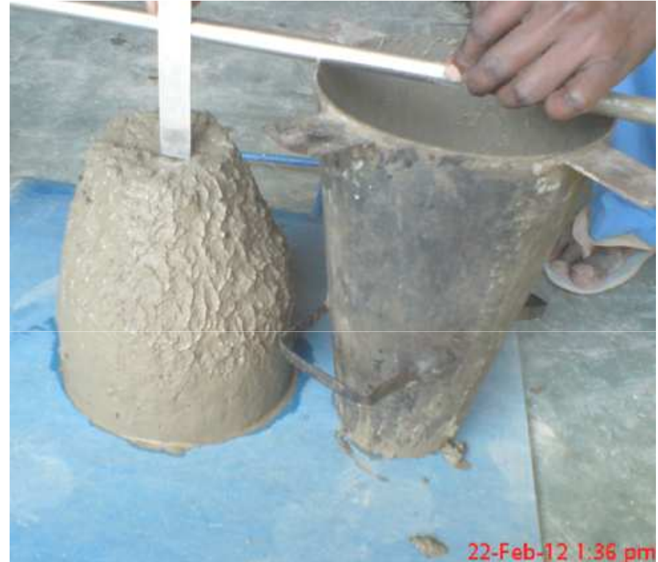
Concrete Slump @ 13:36 = 90mm
