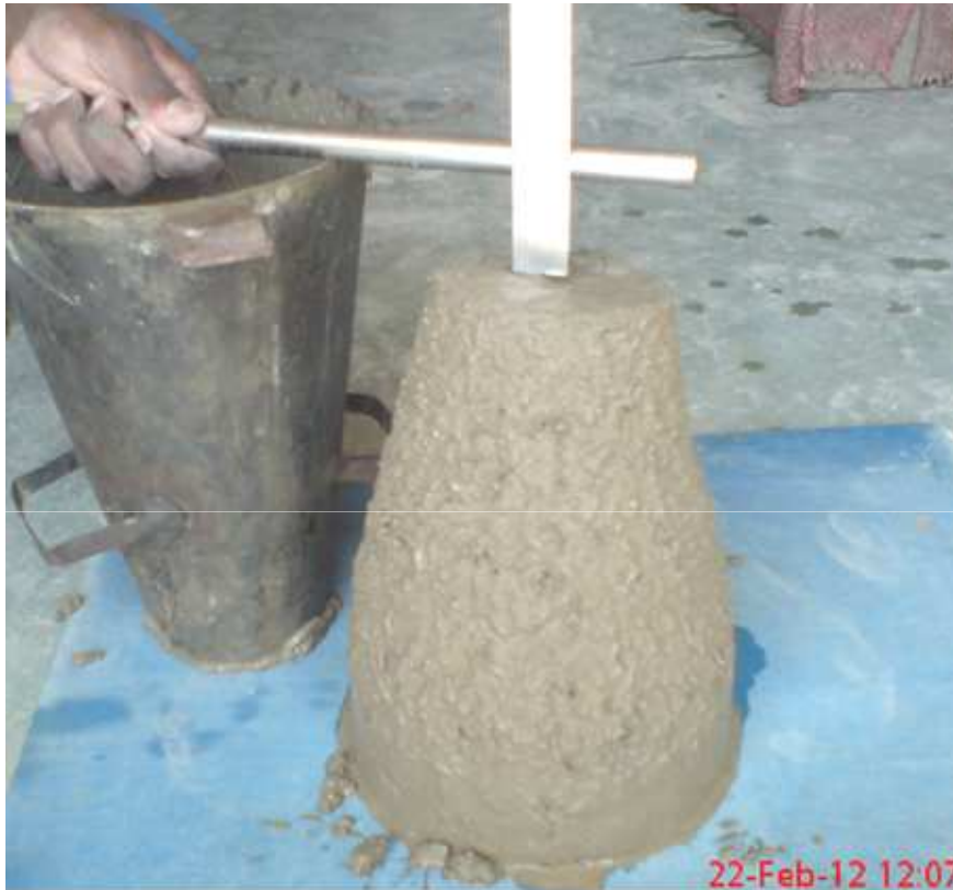
Concrete before Addition of Admixture
