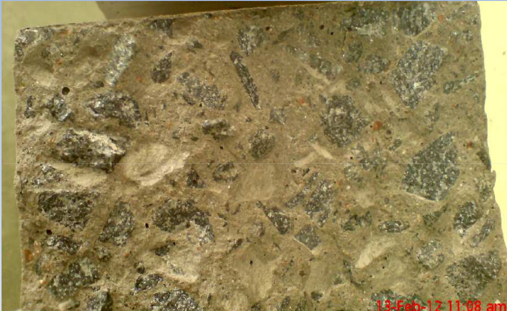
Entrapped Air in M45 Grade Concrete (Fly Ash blended) – Section of well compacted & cured cube
